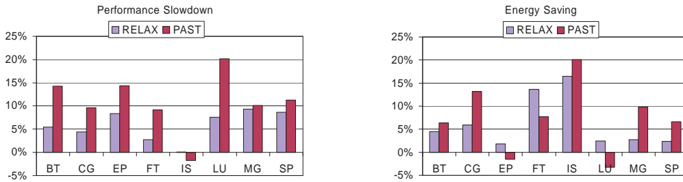
Figure 3. Performance slowdown and energy saving of CPU MISER when using the PAST algorithm and the EMA algorithm with \lambda = 0.5 .
