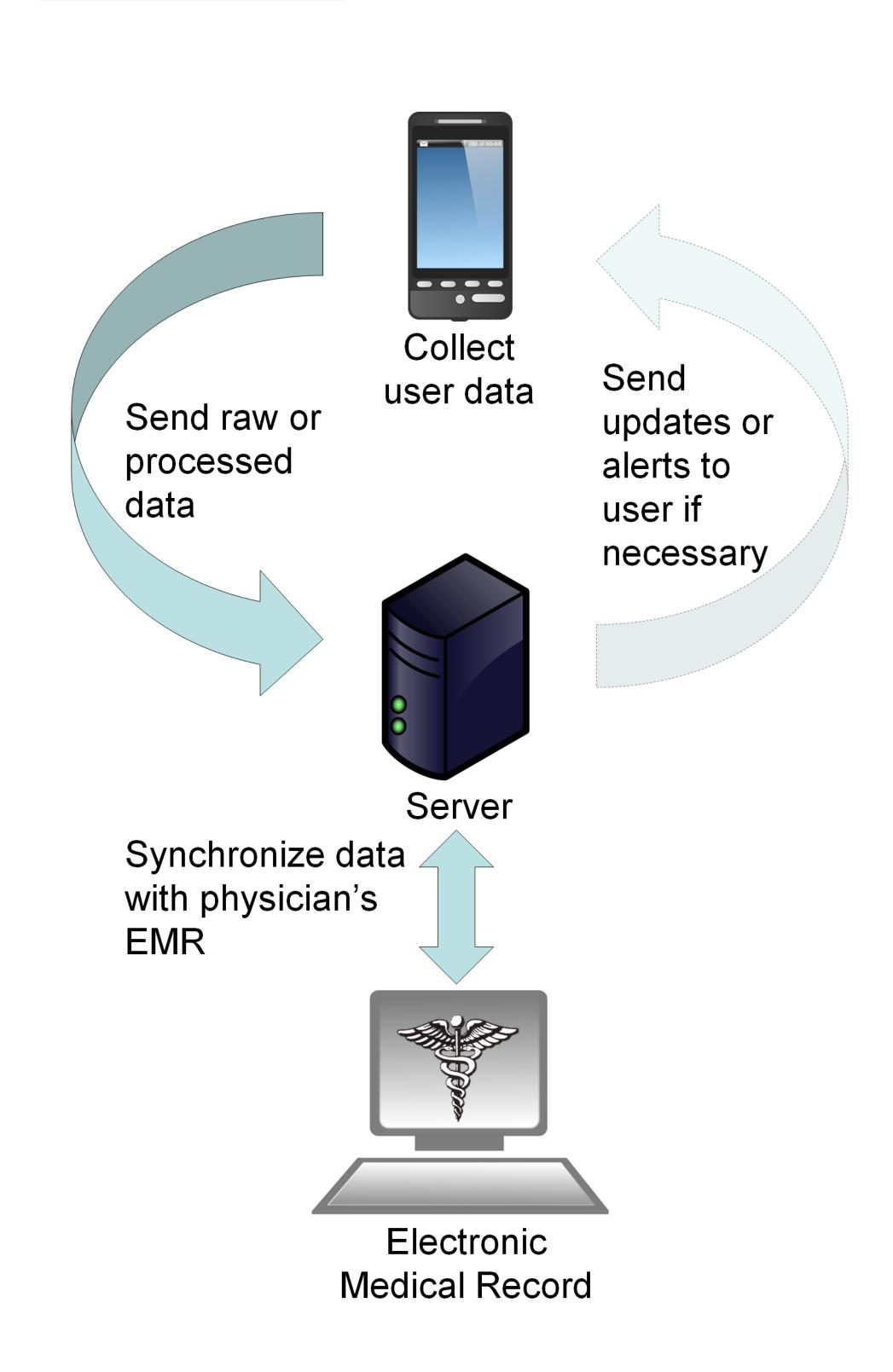
Figure 1: Prototype system architecture
