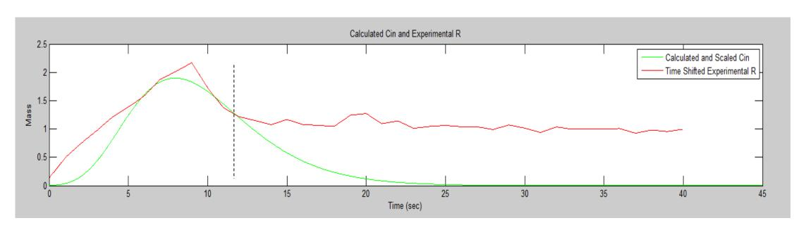
The function that describes the amount of tracer inputted to the system at each time step is not recorded experimentally but is a vital part of the model. We fit a random walk function [1] representing the input function to an initial segment of the experimental mass data curve to obtain Cin(t).
